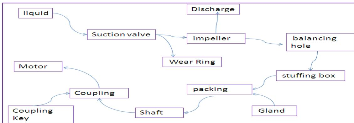
Figure 2. Inter-relationship between the different parts of a centrifugal pump
