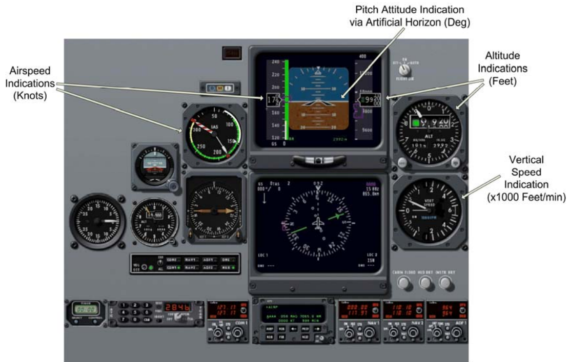
Figure 5: Typical instrument panel showing airspeed, vertical speed, altitude and direction indicating instruments
