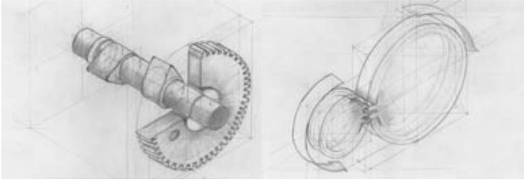
Figure 1 Student drawing: Isometric camshaft with gear ratio
