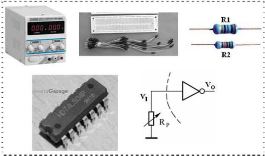
Figure 3. Devices and test circuit used in load characteristic experiment
