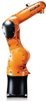
Figure 2. KUKA robot Model KR 6 R700 five (KR AGILUS) with 5 DOF
